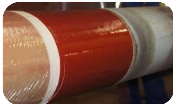
*Resichem 530 HA100 was trialled for a large overseas field joint coating contract by a UK based contractor. The steel pipe was abrasive blast cleaned to SA2.5 surface cleanliness and a minimum 75 micron profile. Resichem 530 HA100 was applied by spray at 300 microns WFT and pory cured at 150-170C in 3 minutes.*
