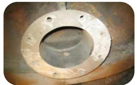
*Corroded bow on large container vessel abrasive blast cleaned and filled using 101 Metal Repair Paste*
