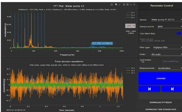
FFT analysis can be performed at each SVT-A sensor. In the figure, the top chart is the FFT waveform, and the bottom chart is the corresponding time-domain waveform. FFT result and time-domain data can be exported to CSV file. Advanced filters can be added for the time domain data and FFT analysis. User can select acceleration or velocity parameters for analysis.
