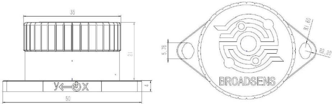
Note: The size of single M6-screw case of SVT-V series sensors is the same as SVT-A series sensors.
